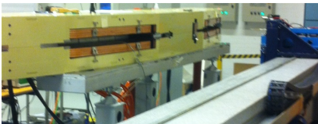
Figure 4: Picture of the prototype 1.5 GeV girder magnetic at our Hall probe field mapping bench.
