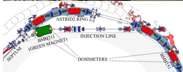
Figure 1: A photo of the ASTRID2 Green Magnet in the beam injection line (top) and a top-view of part of ASTRID2 and its injection line, where the original resistive magnet with coil ends are visible (bottom).
