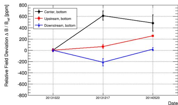
Figure 2: Teslometer measurements at 3 reference points. The data points are relative to the first measurement.
